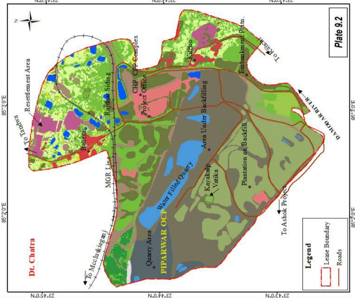
Figure 8.4: Land reclamation status based on satellite data of Piparwar OC, CCL for 2021
