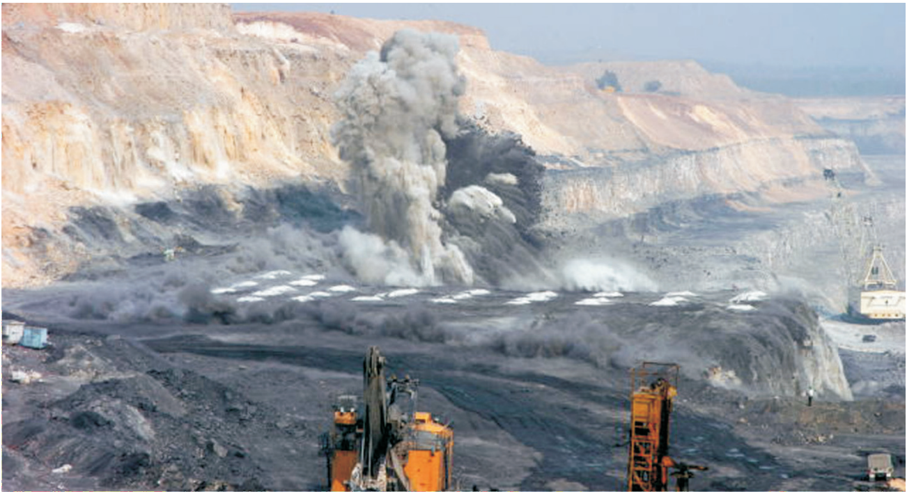
Heavy blasting before coal extraction, in an opencast coal mine
