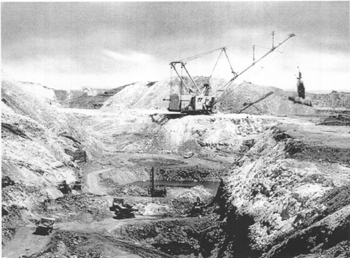
A large Dragline is in operation during OB removal activity in an opencast coal mine.
