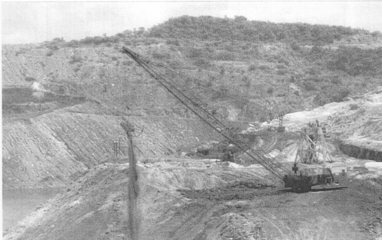
A broad view of a coal face with Large Dragline in over burden removal operation, green plantation over OB Dumps seen in the backdrop
