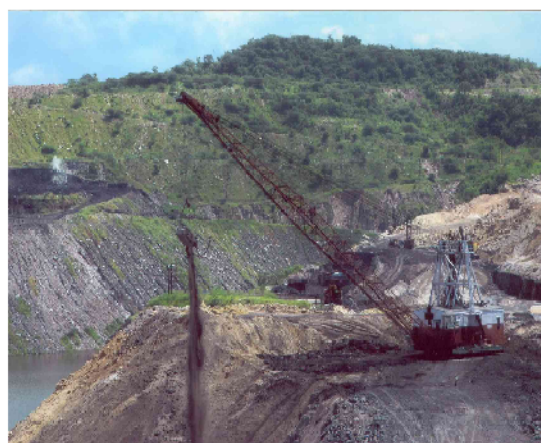
A broad view of a coal face with Large Dragline in over burden removal operation.
