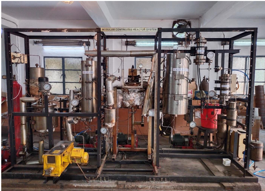
BENCH SCALE WATER GAS SHIFT REACTOR
