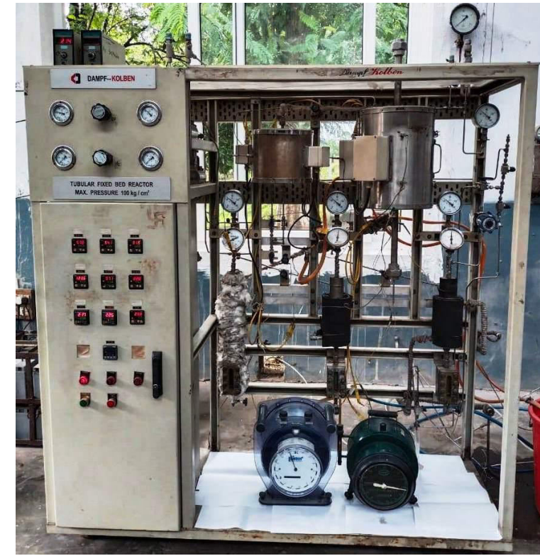
SYNGAS TO METHANOL REACTOR
